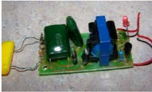
Figure – Electric shock boost circuit
